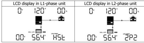
Step 4: Switch on all AC breakers of Line wires in AC input. If AC connection is detected and split phases are matched with unit setting, they will work normally. Otherwise, they will display warning 15/16 and will work in the line mode.
