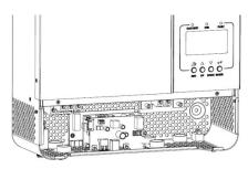
**Step 8:** Put wire cover back to the unit. Now the inverter is providing parallel operation function.
