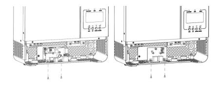
**Step 3:** Remove two screws as below chart and remove 2-pin and 14-pin cables. Take out the board under the communication boards.
