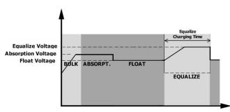
However, in Equalize stage, when battery equalized time is expired and battery voltage doesn't rise to battery equalization voltage point, the charge controller will extend the battery equalized time until battery voltage achieves battery equalization voltage. If battery voltage is still lower than battery equalization voltage when battery equalized timeout setting is over, the charge controller will stop equalization and return to float stage.
