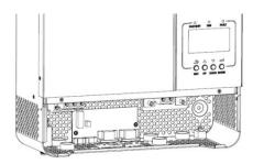
**Step 6:** Re-connect 2-pin and 14-pin to original position of parallel board, and re-connect 2-pin and 6-pin to original position of communication board.
