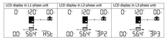
Step 4: Switch on all AC breakers of Line wires in AC input. If AC connection is detected and three phases are matched with unit setting, they will work normally. Otherwise, they will display warning 15/16 and will not work in the line mode.
