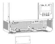
**Step 4:** Remove two screws as below chart to take out cover of parallel communication.
