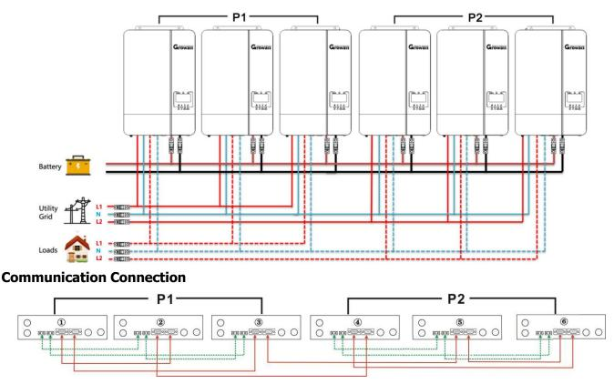
**WARNING:** Do not connect the current sharing cable between the inverters which are in different phases.
