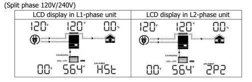
Step 5: If there is no more fault alarm, the system with split phase output is completely installed. Step 6: Please switch on all breakers of Line wires in load side. This system will start to provide power to the load.
