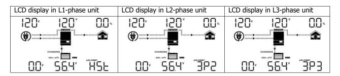
Step 5: If there is no more fault alarm, the system to support 3-phase equipment is completely installed. Step 6: Please switch on all breakers of Line wires in load side. This system will start to provide power to the load.
