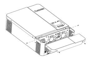
**Step 2:** Remove WiFi/GPRS communication board and CAN/RS485 communication board by unscrewing screws as below chart, and remove 2-pin and 6-pin cables.
