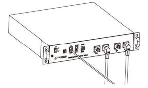
**Note:** If choosing lithium battery, make sure to connect the BMS communication cable between the battery and the inverter. You need to choose battery type as "lithium battery".
